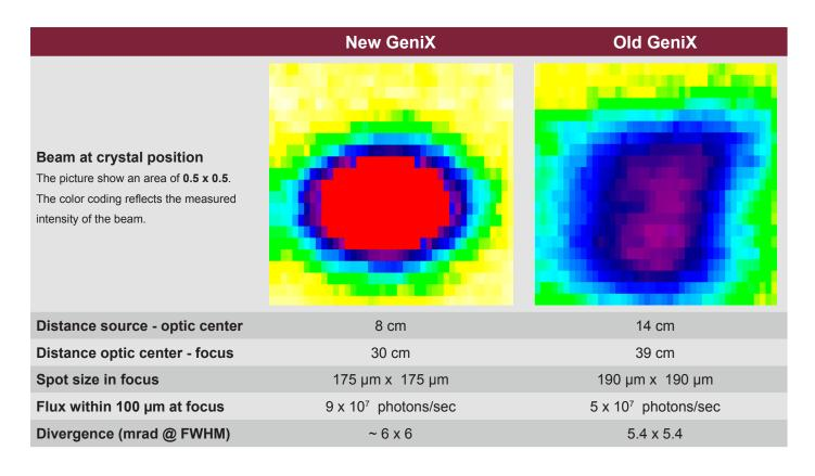
Comparison of the GeniX 3D Cu HF beam delivery system with the Genix Cu VHF system
