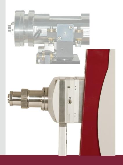
Comparison of the GeniX <sup>3D</sup> Cu HF beam delivery system with the GeniX Cu VHF system
